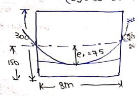
a) detection due to prestressing force (posabolic eccent eity tons
