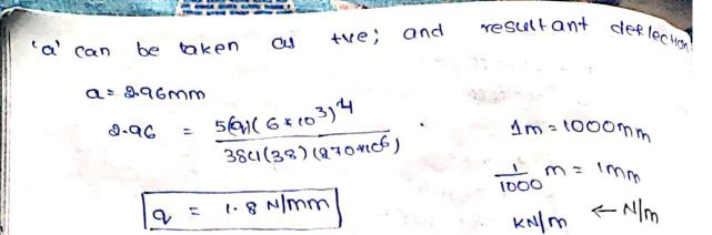
3) A rectangular beam of cls section 150mm & 300mm deep is simply supposed over a span of 8m & is prestressed by means of a symmetric parable cable at a distance of 75mm from the bottom of the beam, at mid span & 125mm from the top of the beam at the support sections. If the force in the Cable is 350km and to = 38 km/mm² calculate: (a) the deflection of mid span when the beam is supporting its own weight.
