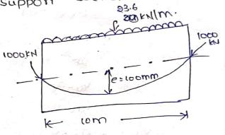
The self-weight of the beam -Areax density of concrete. 10.9540.649U
